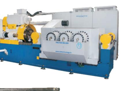
125T - Twin Head Machine One head fixed and the other moving for simultaneous welding at both ends
