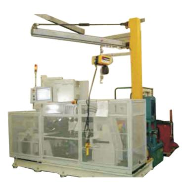
This is a computerized standalone system to perform hub rotational durability test operations with block programming and controlled parameters.
