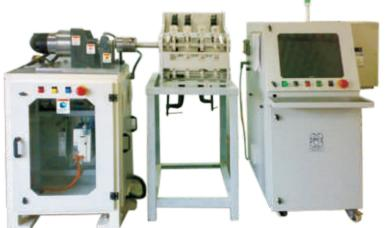
This test rig facilitates endurance test requirements on all accelerator pedal modules.
