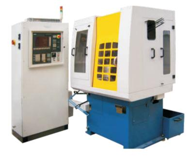
The valve is held on the stem by a collet in a special spindle and two tools on a two-axis CNC slide form or generate the groove and chamfer. Tappet face is also machined in the same setting. The jobs are automatically loaded and unloaded. Cycle time achieved is less than 10 seconds.
