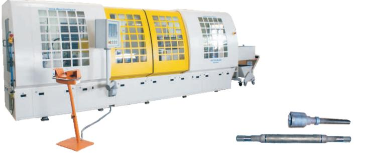
Designed for welding Stub Shaft / Tripod to Tubular Shaft
