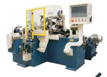
Designed for welding Engine Valves - Head to Pin
