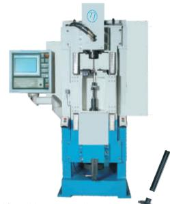
Designed for welding Engine Valves Forged Head to Pin Max. forge force Max. dia. at weld
