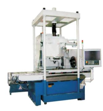
This three-axis vertically configured Friction Stir Welding machine accommodates a maximum plate size of 1000mm x 400mm and has a maximum thrust of 100 kN on Z- axis.
